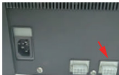
8. Connect the cable to the milk cooler (other connector is optional)
